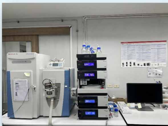
Ultra high performance liquid chromatography coupled with high resolution mass spectrometer, LC-MS
